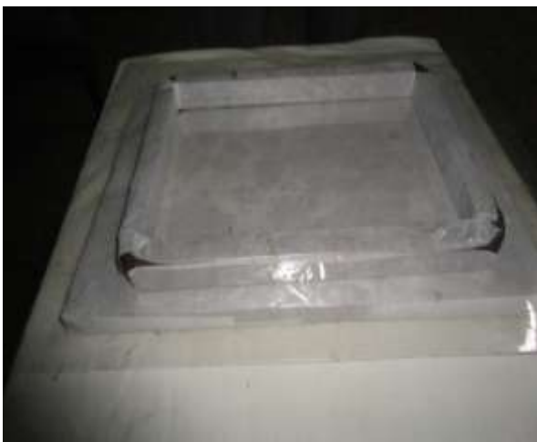
Fig 2:Hand Lay-up Method
