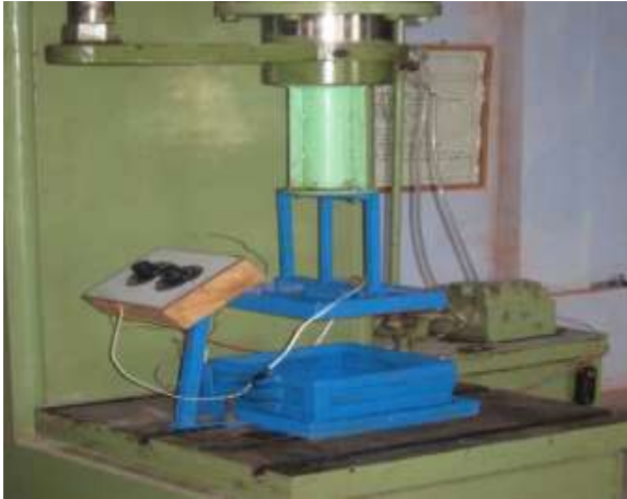
Fig 1:Compression Moulding Machine
