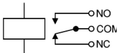
The relay's switch connections are usually labeled COM, NC and NO:
