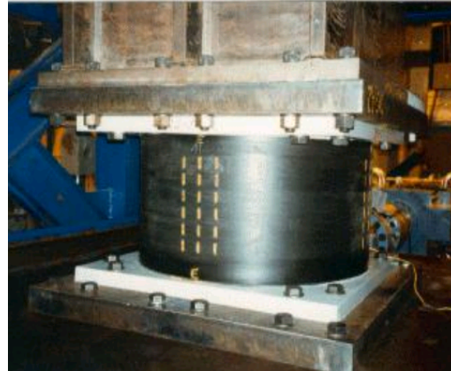
(Fig:3) actual picture of base isolation in a building.
