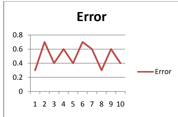
Fig.6 Chart showing Error between Thermometer Reading and LM 35 Reading in °C
