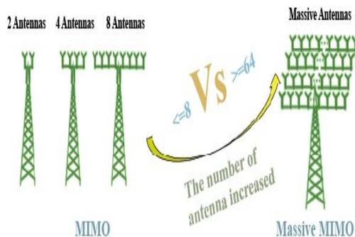
Fig. 3 MIMO vs. Massive MIMO
