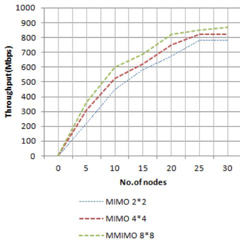
Fig. 6 Throughput describing the successful transmission of packets w.r.t various techniques
