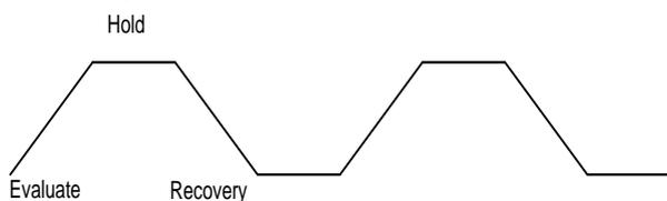
Fig.1. Four Phased Trapezoidal Power Clock
