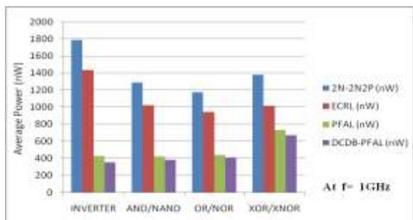
Fig.9. Graph showing average power dissipation for different logic gates using proposed DCDB-PFAL, ECRL, 2N-2N2P, PFAL at 1GHz
