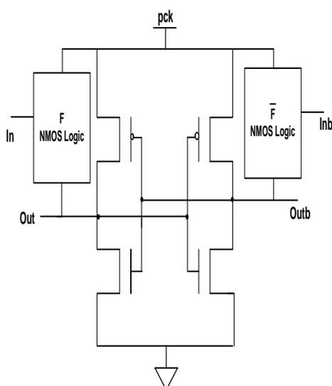
Fig.4. PFAL Basic logic circuit
