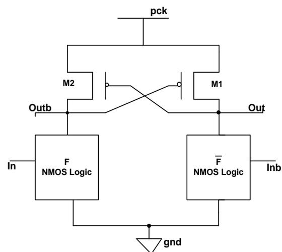
Fig .2. Efficient Charge Recovery Logic (ECRL)
