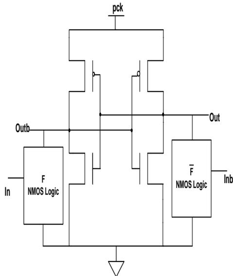
Fig .3. 2N-2N2P Basic Logic circuit
