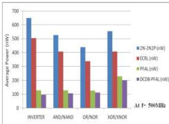
Fig.8. Graph showing average power dissipation for different logic gates using proposed DCDB-PFAL, ECRL, 2N-2N2P, PFAL at 500MHz
