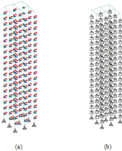
The Structure Model of Group of 9 piles after being assigned with (a) Elastic Soil springs (b) Multi linear Soil Springs
