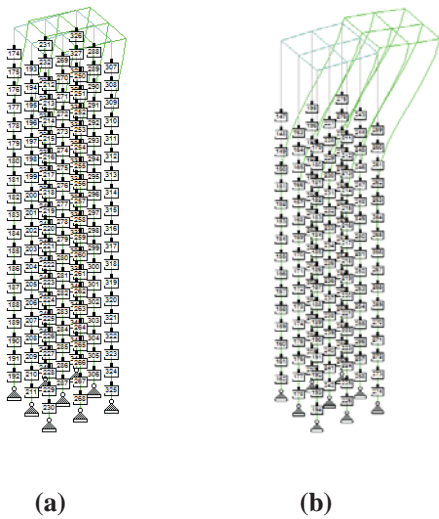
Comparison of Lateral Displacement of the Pile Group (a) Interior Pile (b) Exterior Pile; at F_t = 1500 kN (337 kips) (the Displacements Are Amplified 100Time)
