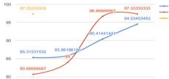
Figure 10 Plot of Mean Arterial Pressure readings taken by Sphygmomanometer Vs the System
