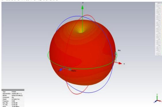
Fig. 6 H-field of antenna @ 5.54 GHz in CST 2016.
