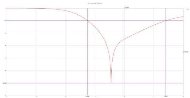
Fig. 2(b) Return loss plot (S11) showing bandwidth of antenna design.
