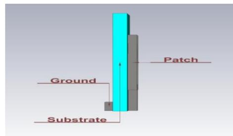
Fig. 1 (a) Lateral view of the propounded antenna design.
