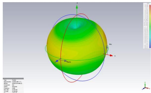
Fig. 4 Directivity of antenna @ 5.54 GHz in CST 2016.
