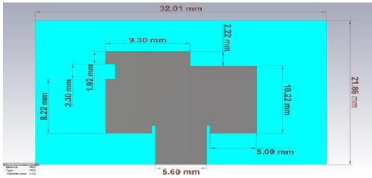
Fig. 1 (b) Top view of the propounded antenna design
