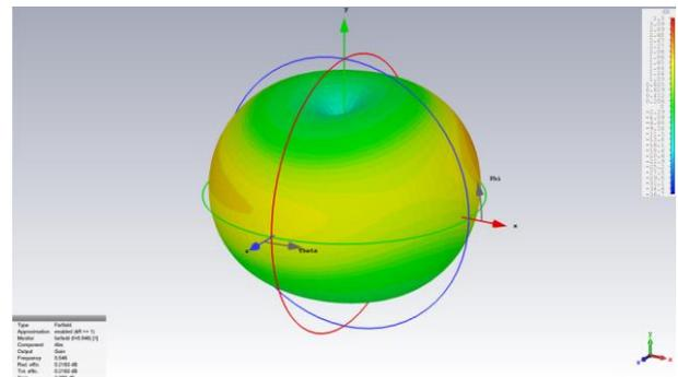
Fig. 3 Gain of antenna @ 5.54 GHz in CST 2016.
