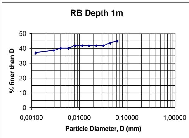
Fig.2: Hydrometer results for samples RC1, RC2 and RB from 1 metre deep.
