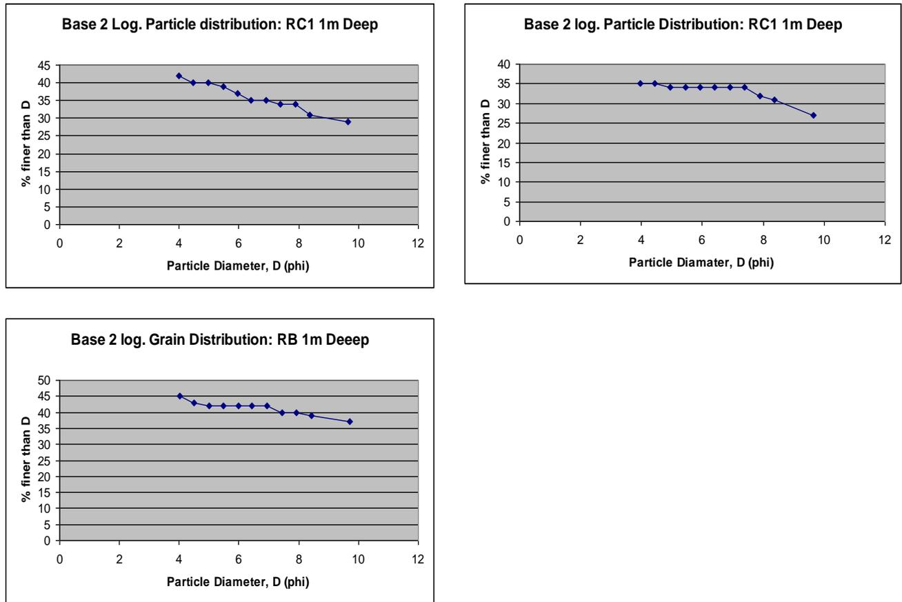
Fig. 3: Base two logarithmic particle size distribution curves for 3 samples.
