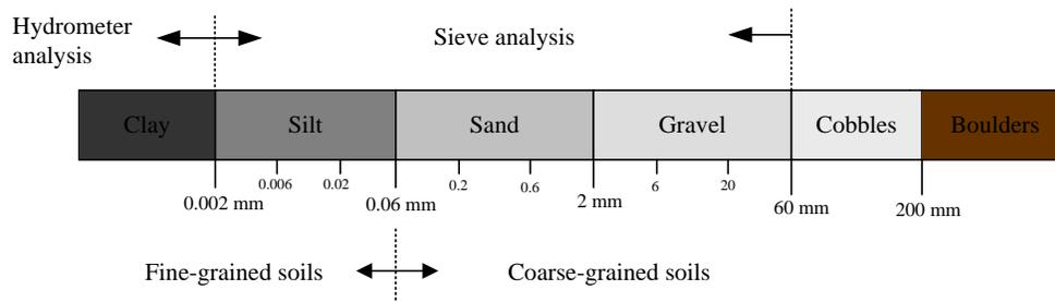
**Fig.1:** Grain size distribution for dry and wet sieve analysis.
