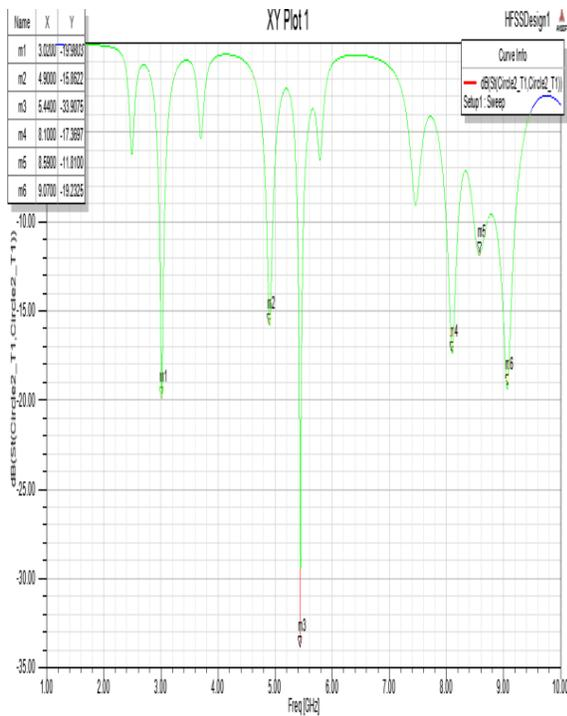
Fig.9 return loss for proposed antenna design [13]
