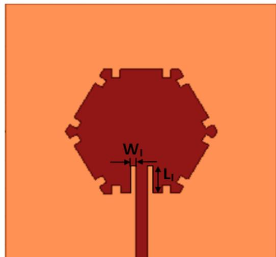
Fig.4 Design of proposed antenna with inset feed [11]
