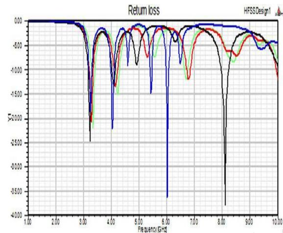
Fig.10 Return loss versus frequency plots for 0<sup>th</sup>, 1<sup>st</sup>, 2<sup>nd</sup> and 3<sup>rd</sup> iterations [14]
