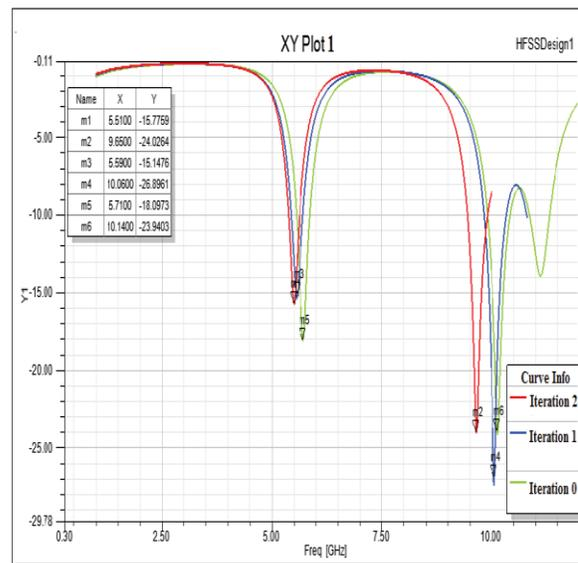
Fig.7 Return loss versus frequency plot of 0<sup>th</sup>, 1<sup>th</sup> and 2<sup>nd</sup> iterations [12]
