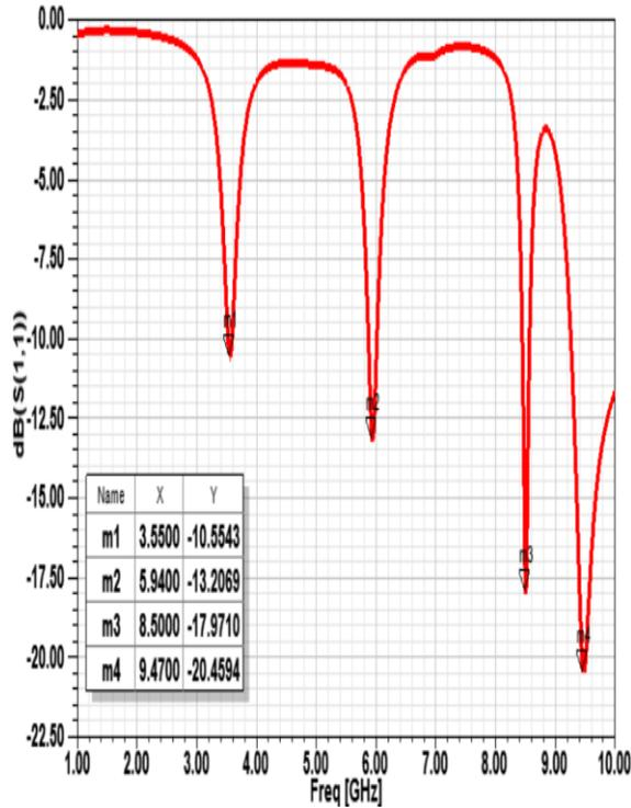
Fig. 5 Return loss curve of proposed antenna with inset feed [11]
