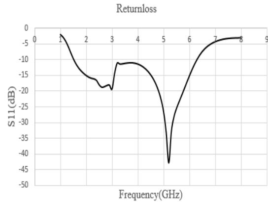
Fig. 3 Return loss of the optimized antenna [10]
