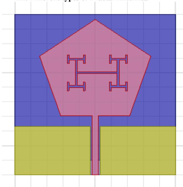
Fig.2 microstrip pentagonal patch antenna with H-Tree with fractal slot [10]
