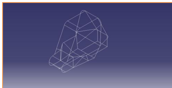
Figure 5: Wireframe model of the roll cage.
