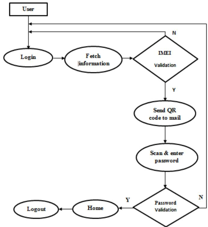
Fig. 2 Flow diagram of user login process
