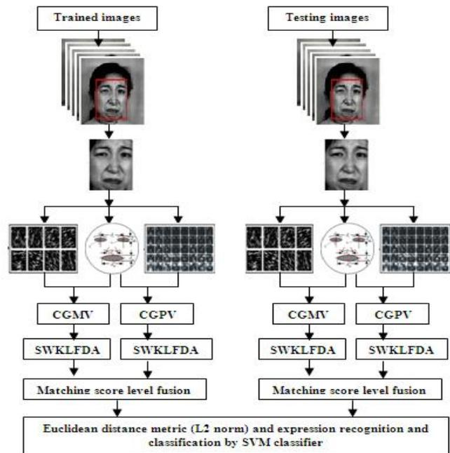
Fig. 1 Schematic diagram of expression recognition system using proposed approach.
