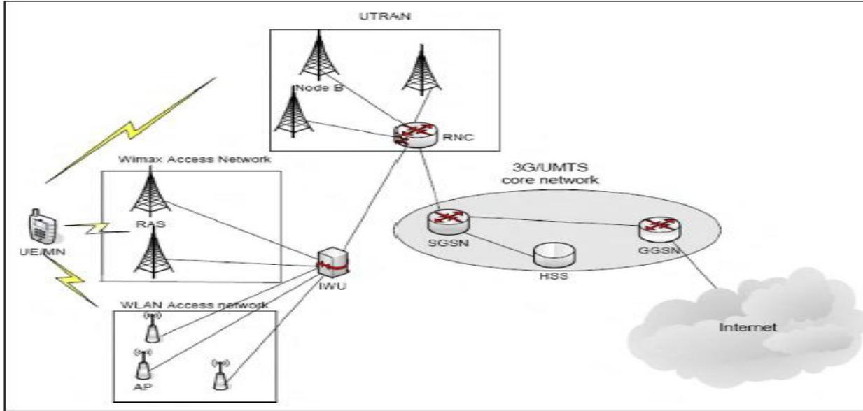
Figure 3: Tight Coupling Integration at RNC Level
