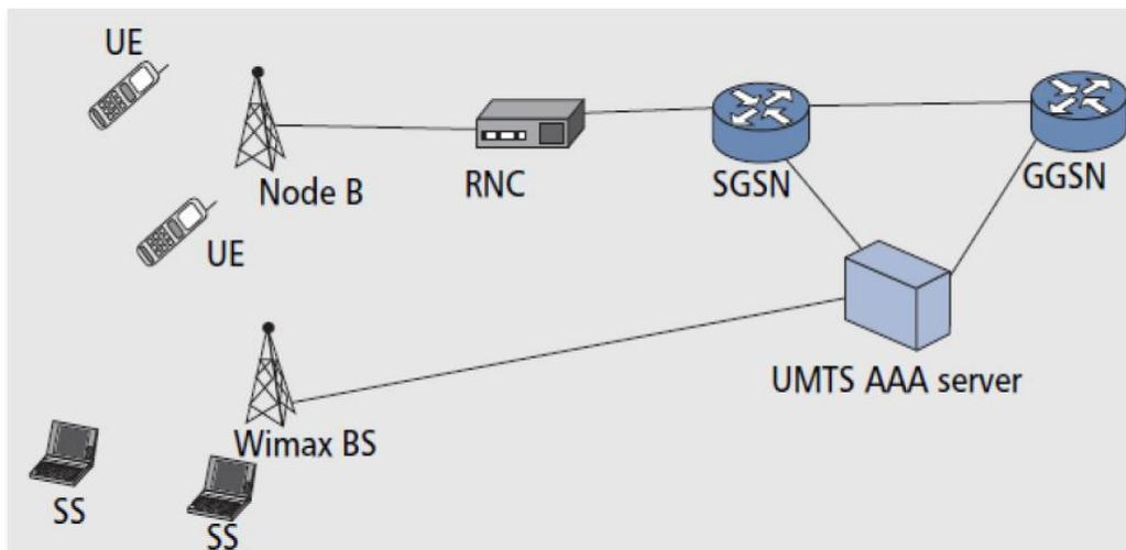
Figure 1: Loose Coupling Integration
