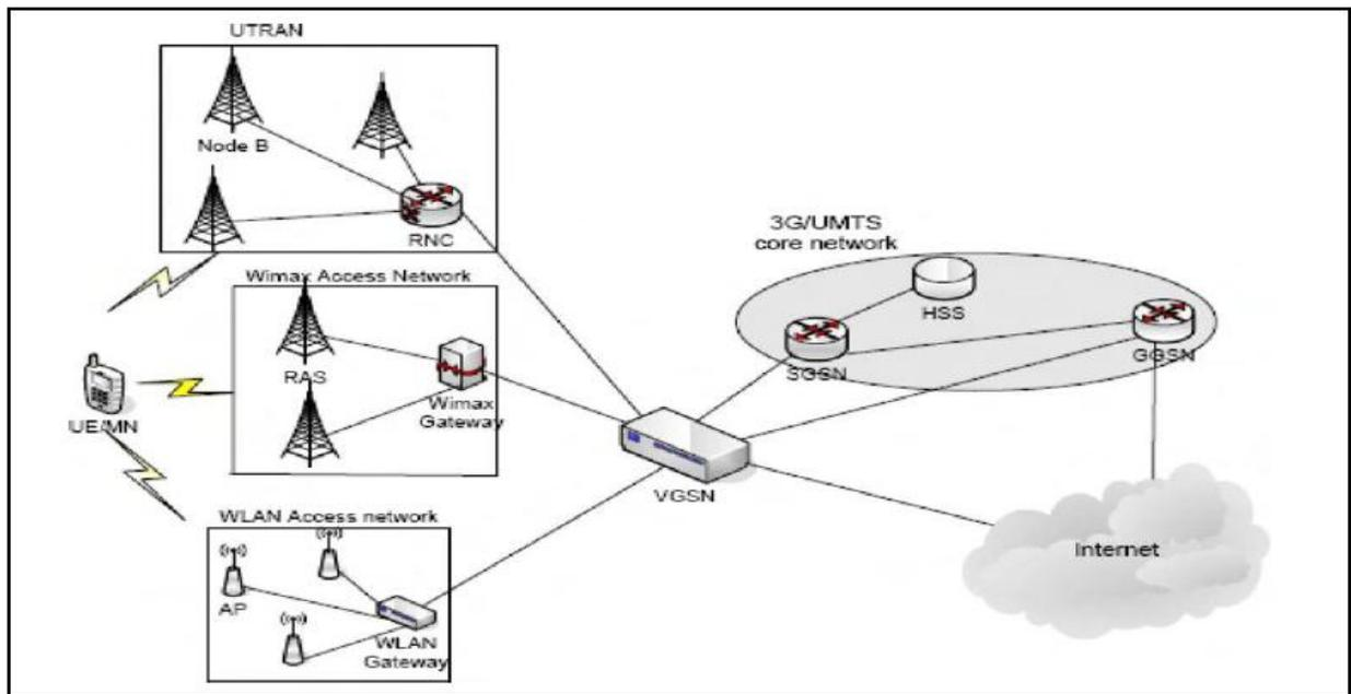
Figure 2: Tight Coupling Integration at GGSN Level
