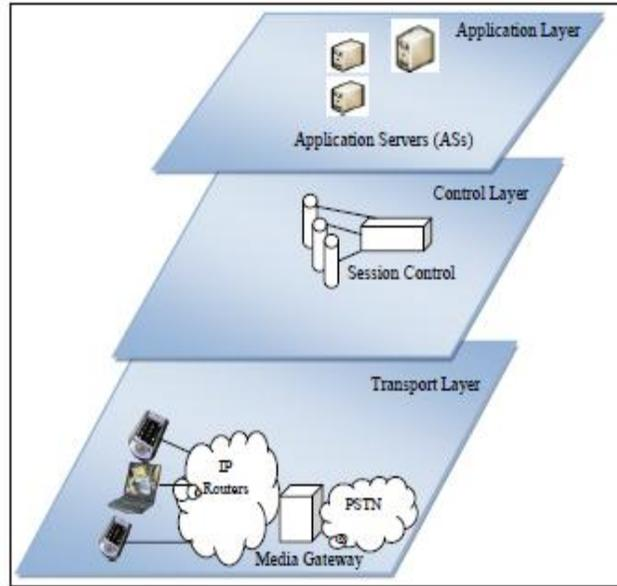
Figure 7: Application, Control and Transport Layers of an IP Multimedia Subsystem
