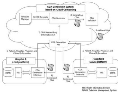
Fig 2.The architecture of CDA generation system
