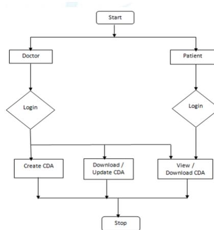
Fig3: data flow diagram
