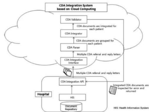
Fig. 1. The architecture of CDA integration system
