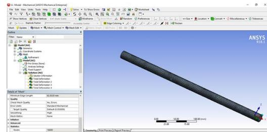
FIGURE 3 Meshed drive shaft in ANSYS 18.1 software
