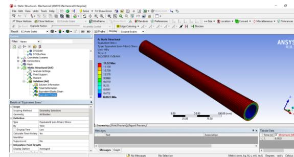
Figure 10 Equivalent elastic stress of carbon composite shaft
