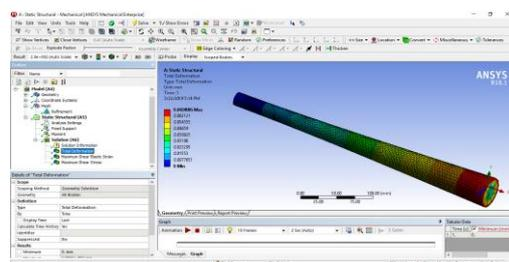
Figure 5 Total deformation of drive shaft
