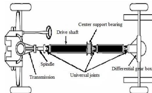
FIGURE 1 CONVENTIONAL TWO-PIECE DRIVE SHAFT ARRANGEMENTS [4]
