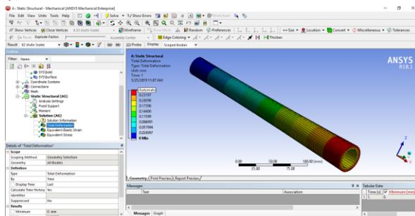
Figure 8 Total deformation of carbon composite shaft
