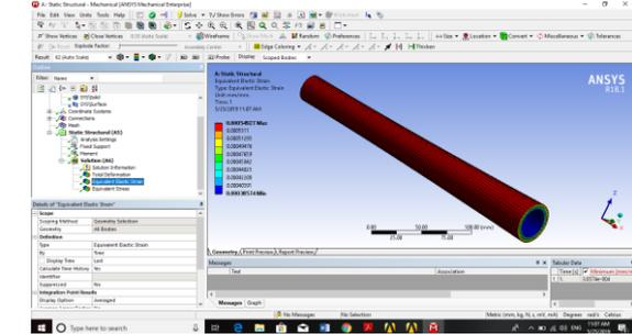
Figure 9 Equivalent elastic strain of carbon composite shaft
