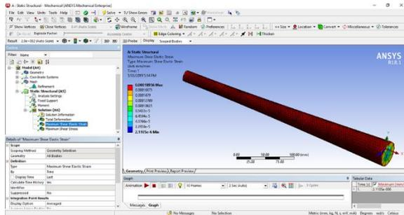
Figure 6 Equivalent elastic strain of drive shaft
