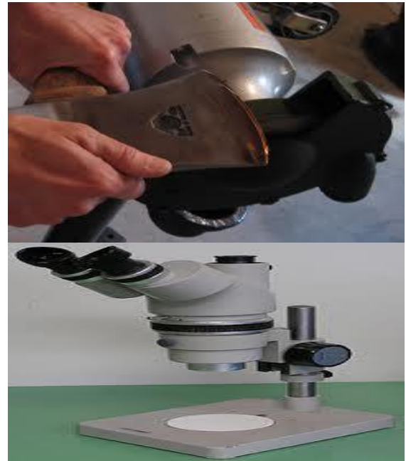
Figure 2.6 Belt Grinder used for polishing and Optical Microscope used for Microstructure examination
