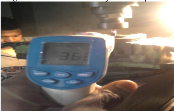
Figure 2.4 Complete Setup while running the VMC & Temp.Measurement
