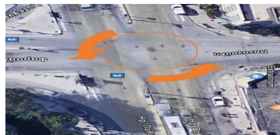
Fig. 3: Increase the length of left-turn lane to avoid the through-lane blocking cause of left-turn traffic demand
