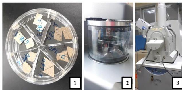
**Fig. 1: The following process for scanning electron microscope (SEM) analysis. 1) Preparation of samples 2) Coating and, 3) SEM analysis.**
