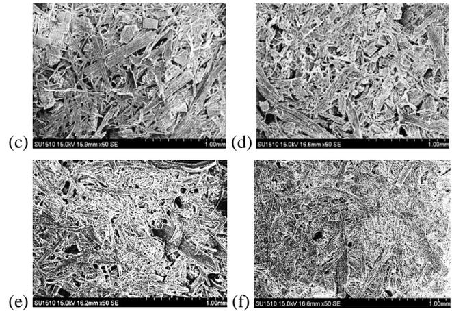
**Fig. 5: Surface morphology (SEM) of oil palm residue handsheet images (50x magnification), (a) OPL untreated, (b) OPL treated, (c) OPT untreated, (d) OPT treated, (e) EFB untreated, and (f) EFB treated.**
