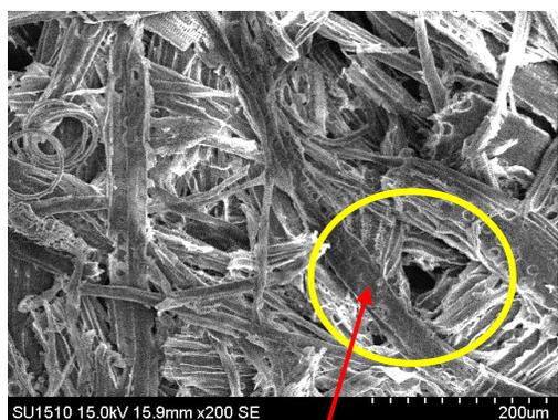
a) The fibre bonds were less and uneven. The fibre size was thicker compared with (b).
