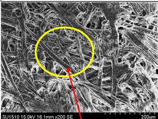
b) The fibre bonds were visible with less gaps. The EFB structure had really great compactness and more evenly fibre size.
