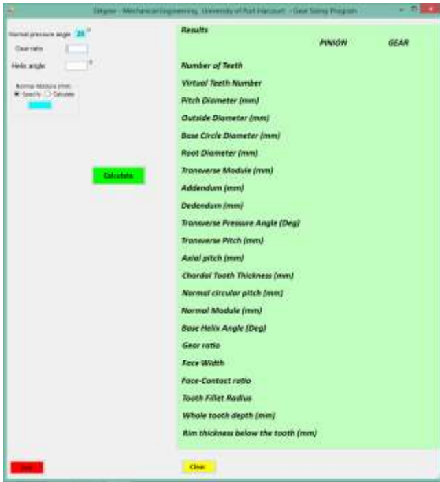
Fig. 3 A screen shot of helical gear sizing interactive user-interface
