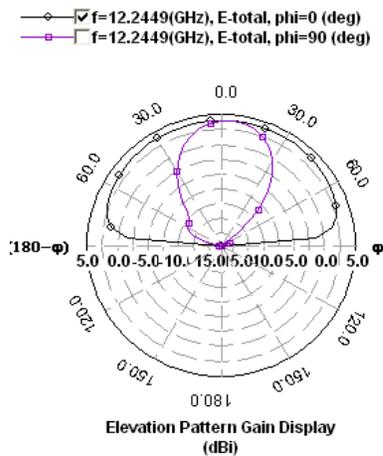
Fig 6. Simulated result: Radiation pattern of bulk silver patch antenna
