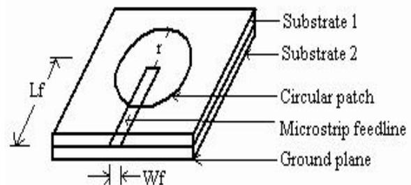
Fig. 1 Geometry of Proximity Coupled Microstrip Patch Antenna
