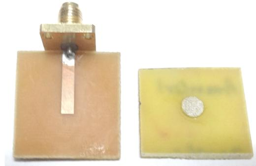
Fig. 4 Fabricated 30 nm thick silver thin-patch proximity coupled antenna. Left: feedline FR4 substrate, right: silver nanofilm patch FR4 substrate
