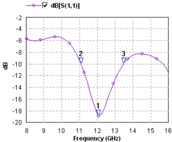
Fig. 3 Simulated response of silver nanofilm antenna: Resonant Frequency vs. Return Loss graph.
