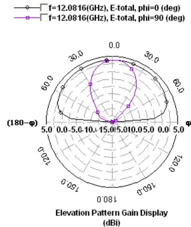
Fig 7. Simulated result: Radiation pattern of silver nanofilm patch antenna
