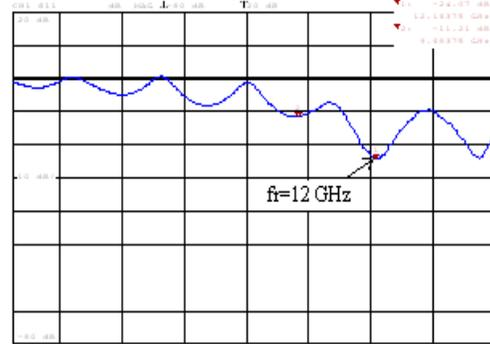
Fig 5. Frequency Response vs. Return Loss graph measured in VNA
