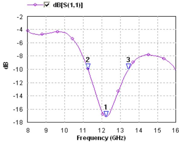
Fig. 2 Simulated response of bulk silver patch antenna: left- resonant frequency vs. Return loss graph, and, right- radiation pattern
