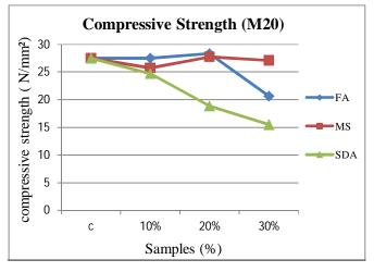
Fig 6. Compressive strength for egg shell powder with admixtures (28 days)
