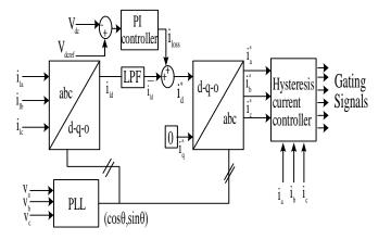
Fig: 4 Gating signals for PWM current controller
