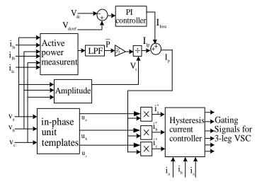
Fig: 5 Gating signals for Carrier less PWM current controller
