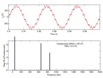
Fig:6 Total Hormin distorsion in output voltage for unbalanced supply voltages
