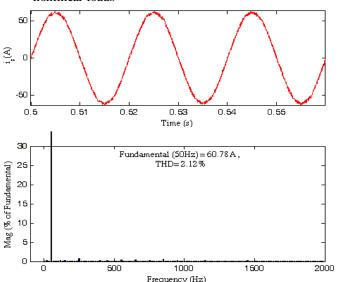
Fig:8 Total Hormin distorsion with active filter
