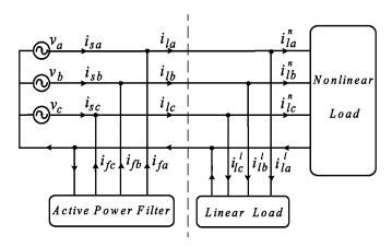
Fig.1. Schematic diagram of three phase four wire shunt active power filter with linear & nonlinear loads
