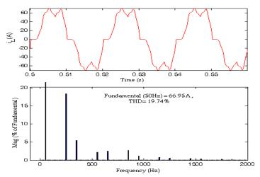
Fig:7 Total Hormin distorsion without active filter for nonlinear loads
