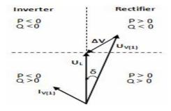
Fig:2 Phasor diagram of VSC and direction of power flows
