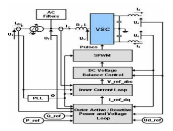
Fig: 3 Overview diagram of the VSC control system
