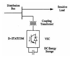
Fig. 1 Schematic representation of the D-STATCOM as a custom power Device [6].
