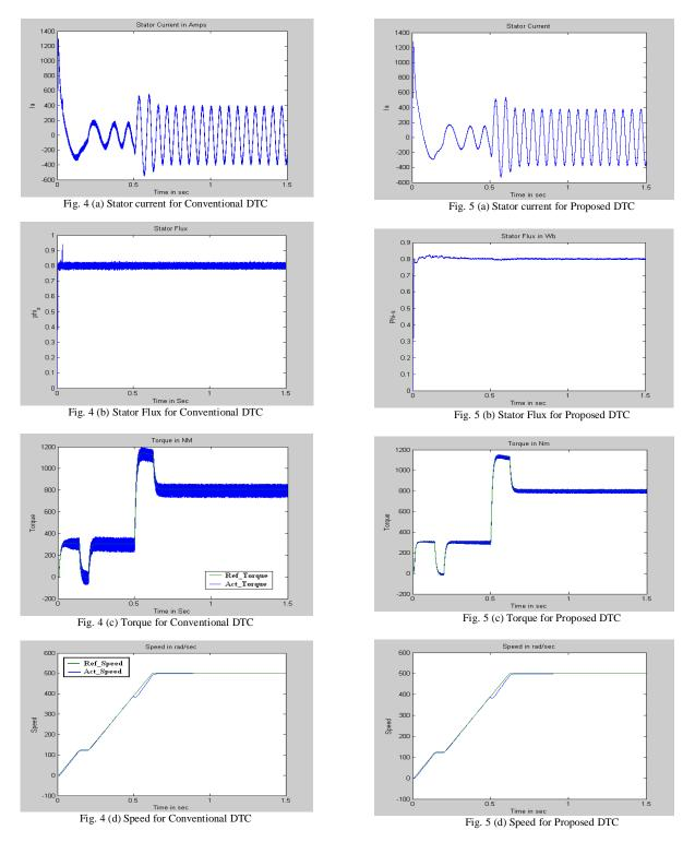
SIMULINK Outputs for Conventional and Proposed DTC - (a) Stator current (b) Stator Flux (c) Torque (d) Speed
