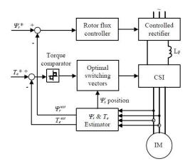
Fig. 1 Conventional DTC CSI-fed IM drive
