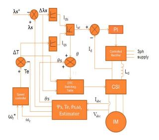
Fig.3 Proposed DTC-SVM Control scheme for CSI fed IM drive
