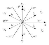
Fig. 2 Sectors in  $\alpha - \beta$  plane where rotor flux resides From the stator output current and voltage, pure integrator in (5) and (6) yields flux vector.
