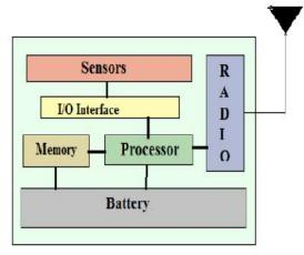
FIG 1. Typical Sensor node
