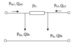
Fig.4. Injection model of the UPFC The admittance  $\begin{array}{c} u\\ Y_m \end{array}$  and  $\begin{array}{c} u\\ Y_n \end{array}$  can be written by [9],
