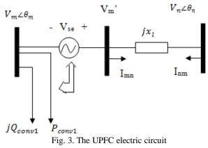
The reactance  $\mathcal{I}$  describes a reactance seen from terminals of the series transformer and is equal to (in p.u. base on system voltage and base power) [11]:
