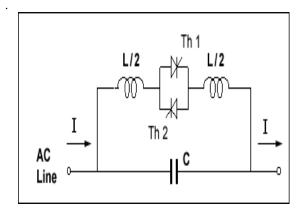
fig 2: thyristor-controlled series capacior(tcsc)
