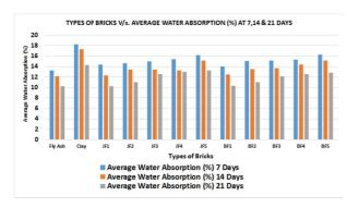
FIGURE 11: TYPES OF BRICKS V/S AVERAGE WATER ABSORPTION (%) AT 7, 14 AND 21 DAYS
