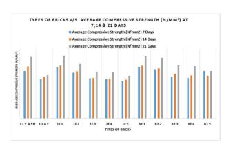
FIGURE 8: TYPES OF BRICKS V/S AVERAGE COMPRESSIVE STRENGTH (N/mm²) AT 7, 14 AND 21 DAYS
