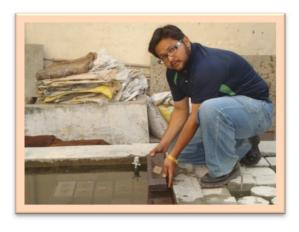
FIGURE 10: CURING OF SAMPLE BRICK
