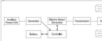
**4. POWERSPLIT HYBRIDS:** It has benefits of combination of series and parallel characteristics. As a result, they have more efficient at lower speed and parallel tend to be more efficient at higher speeds. Some of the examples of power-split hybrids are Ford, Lexus, Nissan and Toyota.
