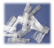
Figure 2: Polypropylene Fiber Source: <u>http://www.google.co.in/images</u>
