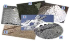
1. Cement, 2. Quarry Dust, 3. Dolomite powder, 4. Polypropylene fibre, 5. Sand, 6. Semi Grit
