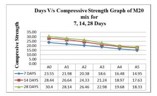
Figure: 3 Percentage Replacement of Ceramic waste V/S Compressive Strength (N/mm<sup>2</sup>) of Concrete for M20 mix at 7, 14 and 28 days
