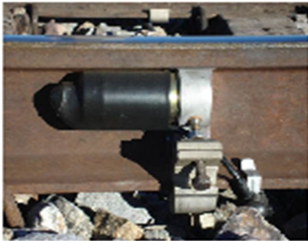
Fig.1 Ultrasonic Broken Rail Detector
