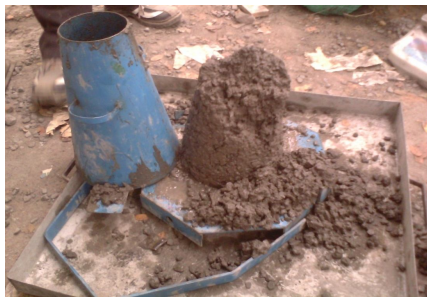
Fig. 1 Slump test performed
