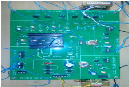
Fig.7 Interfacing of Arduino with PS21765 Intelligent Module
