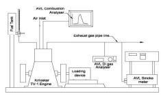
Fig 1 Test Engine
