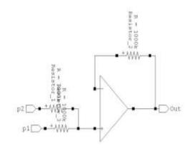
Fig.3: Schematic diagram of Adder
