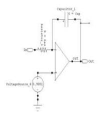
Fig.2: Schematic diagram of Integrator
