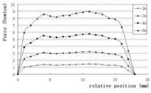
Fig.6 Force output of propulsion phase
