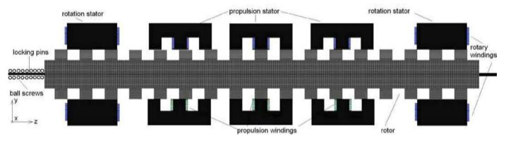
Fig.1: Layout of the 2D motor
