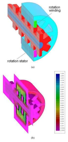
Fig.3 Structure of the rotary motor (a) and flux distribution (b)
