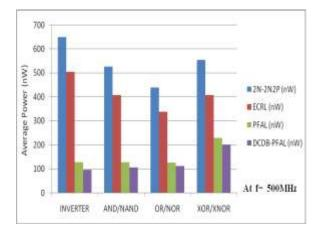
Fig.8. Graph showing average power dissipation for different logic gates using proposed DCDB-PFAL, ECRL, 2N-2N2P, PFAL at 500MHz
