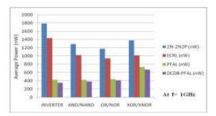
Fig.95. Graph showing average power dissipation for different logic gates using proposed DCDB-PFAL, ECRL, 2N-2N2P, PFAL at 1GHz
