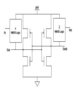
Fig.4. PFAL Basic logic circuit
