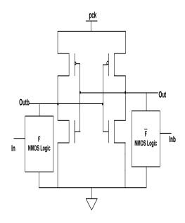
Fig .3. 2N-2N2P Basic Logic circuit
