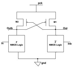
Fig .2. Efficient Charge Recovery Logic (ECRL)
