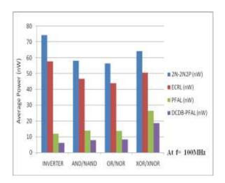
Fig.7. Graph showing average power dissipation for different logic gates using proposed DCDB-PFAL, ECRL, 2N-2N2P, PFAL at 100MHz
