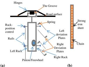
Figure 1. (a) The rack system and flexible speed bump made of plates joined using hinges (b) Chain clamped inside a U-shaped strong iron sheet to make a rack
