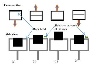
Figure 5. a cross-section and side view showing the position of the rack head in the groove when (a) rack is moving downward (b) rack changing direction at the lowest point (c) rack moving upward (d) rack changing direction at the uppermost point
