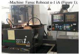
Fig. 1: Wire-cut electrical discharge machine
