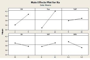
Fig. 2: Main effects plot for surface roughness
