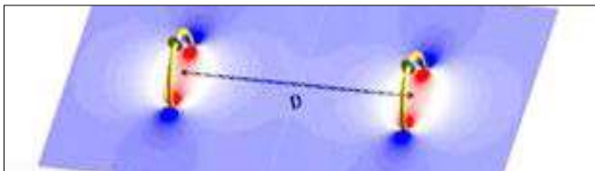
Fig. 8. Simulation Model using Resonant Magnetic Coupling.
