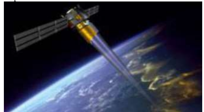
Fig. 4. Example of European Space Agency Aeolus Satellite with laser beam pointing at the Earth's atmosphere. Credits: ESA/AOES Medialab.
