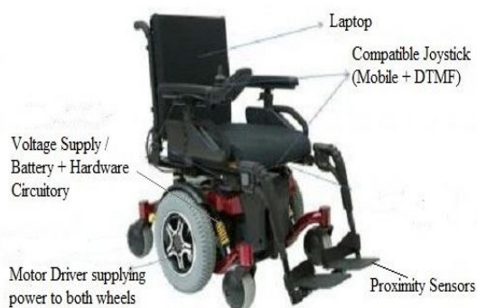
Fig. 3: Cellular Phone controlled Wheelchair
