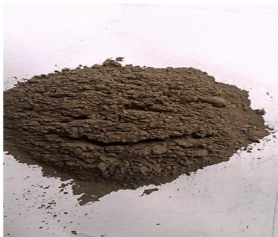
Fig2. Saw Dust Ash
