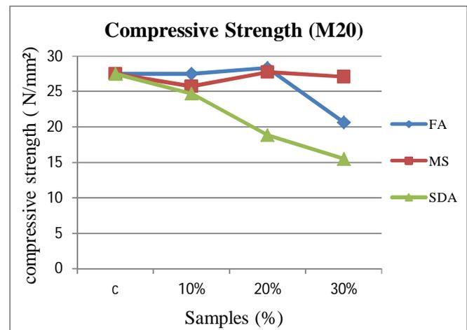
Fig 6. Compressive strength for egg shell powder with admixtures (28 days)
