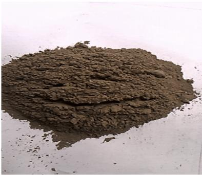
Fig2. Saw Dust Ash
