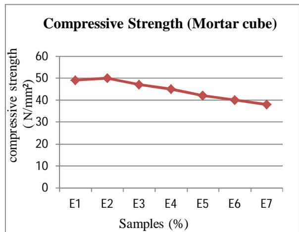
Fig 5. Compressive strength for egg shell powder (28 days)
