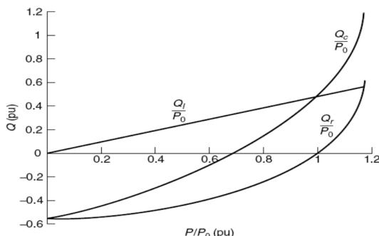
**Figure. 6** The reactive-power flows at the receiving end.
