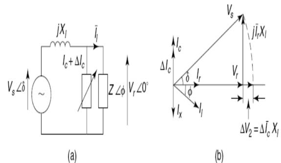
**Figure. 3** The reactive-power control for voltage regulations.
