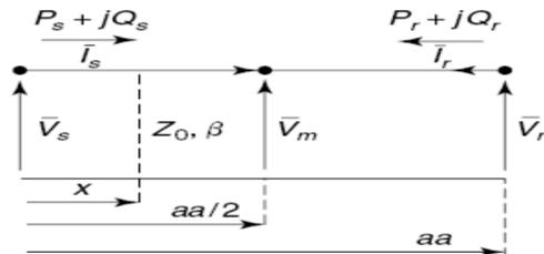
Figure. 4 The power on a lossless distributed line.
