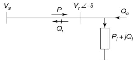
**Figure. 5** The reactive-power balance at the receiving end.
