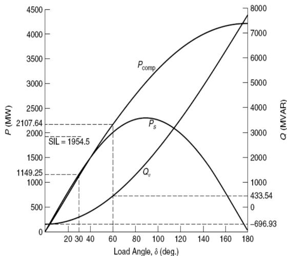
**Figure. 10** The relationship between active power, P, and reactive power, Q, with load angle  $\delta$  in the 735-kV midpoint-compensated line.
