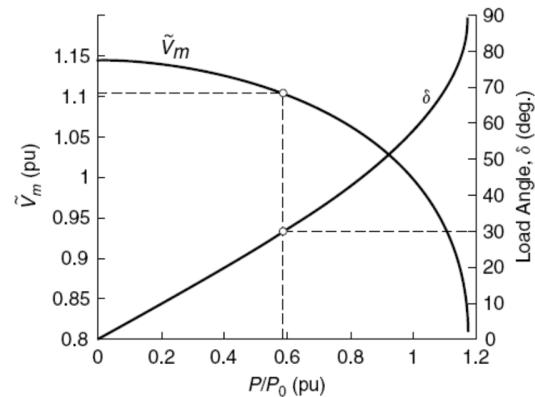
**Figure. 8** The midpoint voltage,  $\tilde{V}_m$ , and load angle,  $\delta$ , as functions of  $P / P_0$ .
