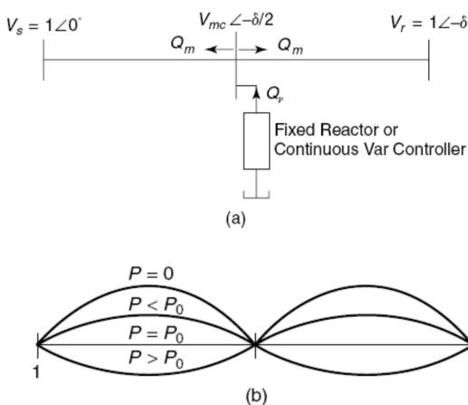
Figure. 9 The midpoint-overvoltage
