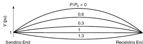
**Figure. 7** The typical voltage distribution on a distributed line.
