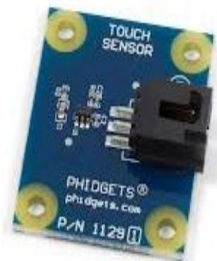
Figure 6: Tactile sensor
