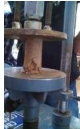
Fig. 2 Failed specimen after UCS test
