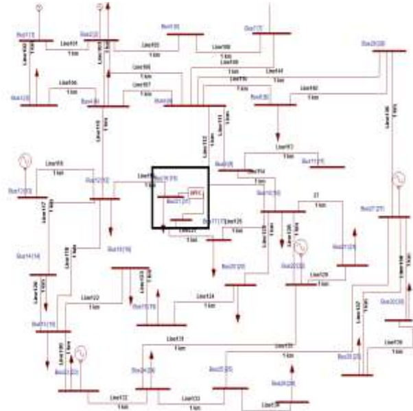
Fig 5: Placement of UPFC
