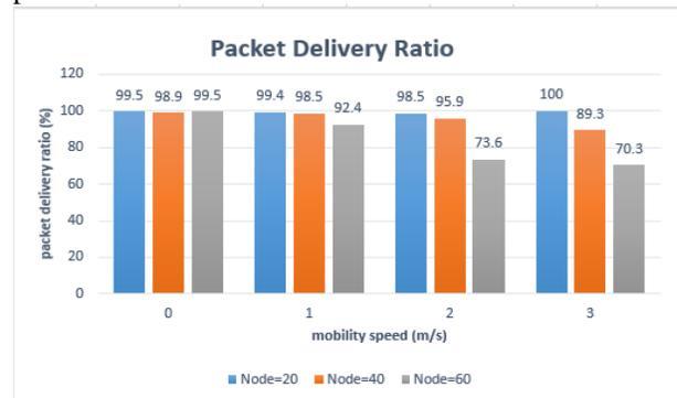
**Figure 7:** Packet delivery ratio at different number of speed and nodes
