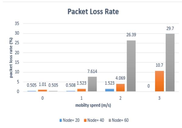
Figure 9: Packet loss rate at different number of speed and nodes
