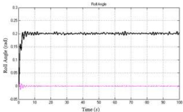
Figure 4. Simulation result of roll angle with SMC
